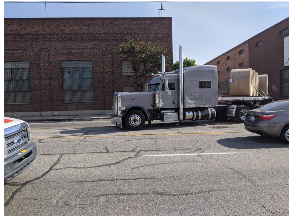
Freight trucks turning onto Santa Fe Avenue require nearly 3 lanes of traffic to effectively make a turn. Directing truck traffic to other corridors as feasible and maintaining roadway design to support these movements are critical considerations.
